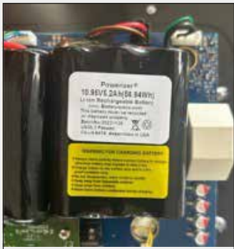
Battery Information There are 2 x packs within a supervisor Unit
