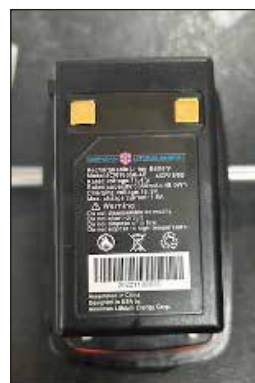
Divers Unit Battery this is 4 in series contained in 1x Unit
