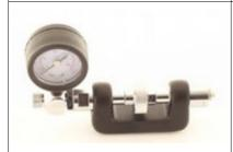
Inline seat adjuster enables the cracking pressure of the ALV and second stage regulators to be adjusted with gas attached.
