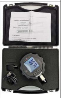
Open Safety IP Gauge (Pressure Gauge) 30 bar. Calibrated. 0.1% FSD
