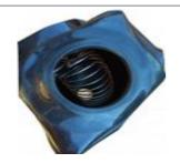
OPV Test Counterlung with pressure bias spring.
